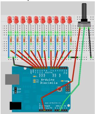
This is the same circuit as in Project 5, but we have simply added the potentiometer and connected it to 5v, Ground and Analog Pin 5.
