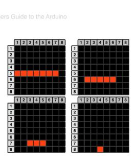
By scanning down the rows and illuminating the respective LED's in each column of that row and doing this very fast (more than 100Hz) the human eye will perceive the image as steady and the image of the heart will be recognisable in the LED pattern.
