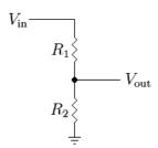
The diagram on the left shows a voltage divider made up of two resistors. The value of Vout will be lower than the value of Vin.
