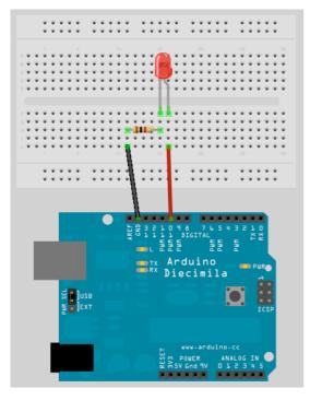
It doesn't matter if you use different coloured wires or use different holes on the breadboard as long as the components and wires are connected in the same order as the picture. Be careful when insterting components into the Breadboard. The Breadboard is brand new and the grips in the holes will be stiff to begin with. Failure to insert components carefully could result in damage.
